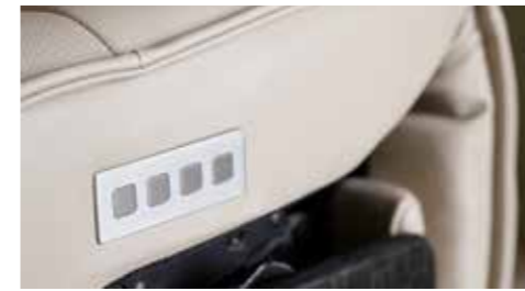
Integrated and concealed control panel placed on the left side of the seat cushion, seen from front.
